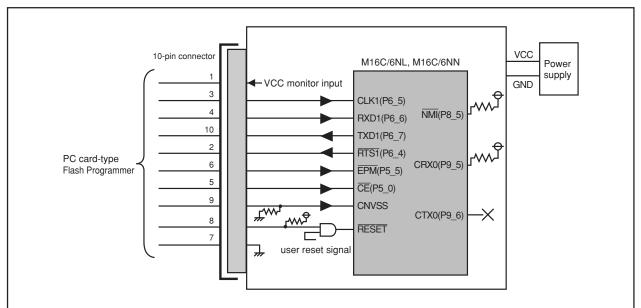
Figure 22.9 Pin Connection for Programming Using Serial I/O Mode
